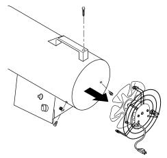
Figure 14 - Removing Motor and Fan Guard from Heater
